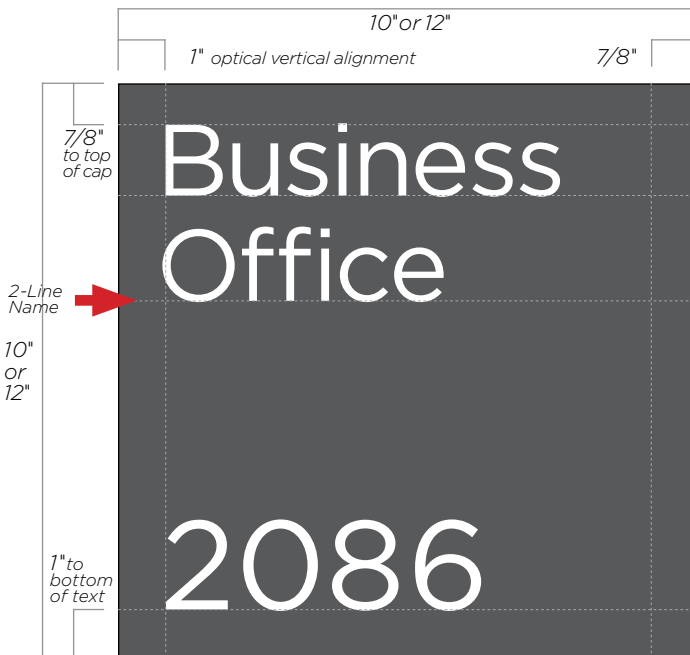
F1, F3 Elevation: 12" x 12" x 3/8" or 12" x 12" x 3/8"
