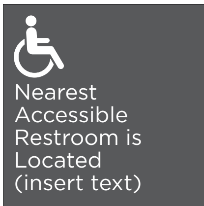
R3B Accessible Restroom Location 7 1/2" x 7 1/2" Minimum text height 5/8" (mounted with non-accessible restroom sign, only used in buildings where there are non-accessible restrooms)
