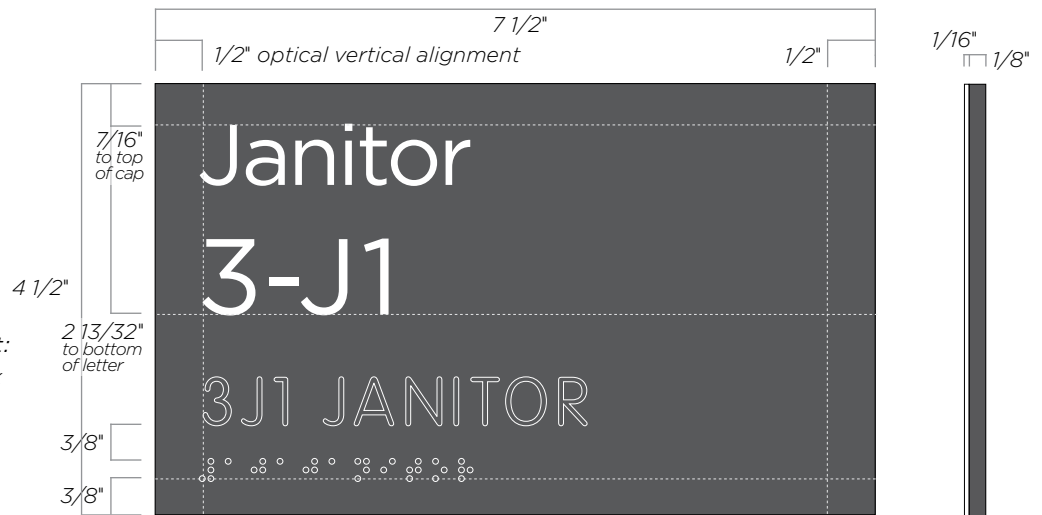
R4 with Room Name, Elevation: 7 1/2" x 4 1/2" x 3/16"
